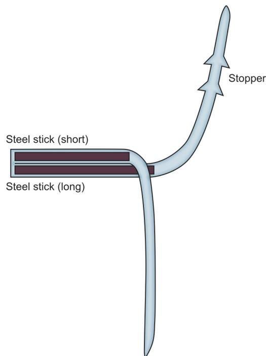
**Fig. 2:** Schema of clamping using gut-clamper: As the two steel sticks are arranged tandem, their gaps is set in the middle of the plastic belt. A distance between these two sticks is 5 mm and the two steel sticks are hooked using the hole (3 mm in diameter) by bending with V-shape at this point
