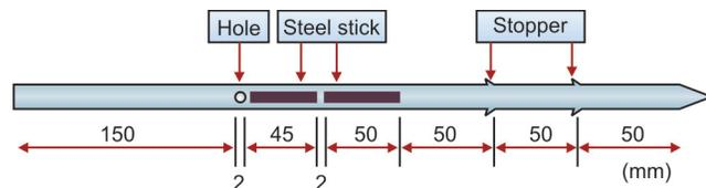
**Fig. 1:** Structure of gut-clamper: Gut-clamper is a 5 mm width, plastic belt of 20 cm long that includes two hard sticks made of stainless steel with a diameter of 3 mm and 40 mm and 45 mm having flexible belts on one ends, a joint at which sticks are joined
